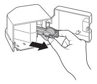
4 Lift an empty **Staple Case** while holding its both edges, then pull out it from the **Staple Cartridge**.
