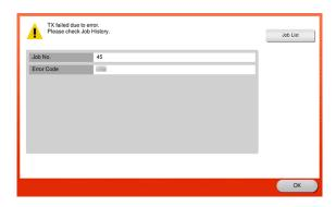
The error code can also be checked on the [Job Details] screen. To display the [Job Details] screen, tap [Job List], select the job that caused the error from [Log], and tap [Details].
