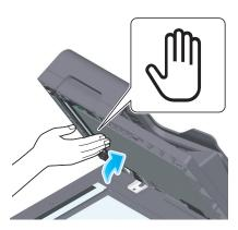
→ Press the Hand mark in the center of the **Opening and Closing Guide**, and check that the **Opening and Closing Guide** is locked securely.
