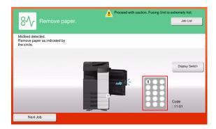
When a paper jam is cleared, a screen showing how to correctly load paper or the original is displayed.
