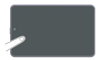
On the Control Panel, press the Power key. If the Weekly Timer setting has put the machine in Erp
