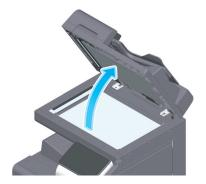
Wipe stains off the Slit Scan Glass using a dry, clean cloth.
